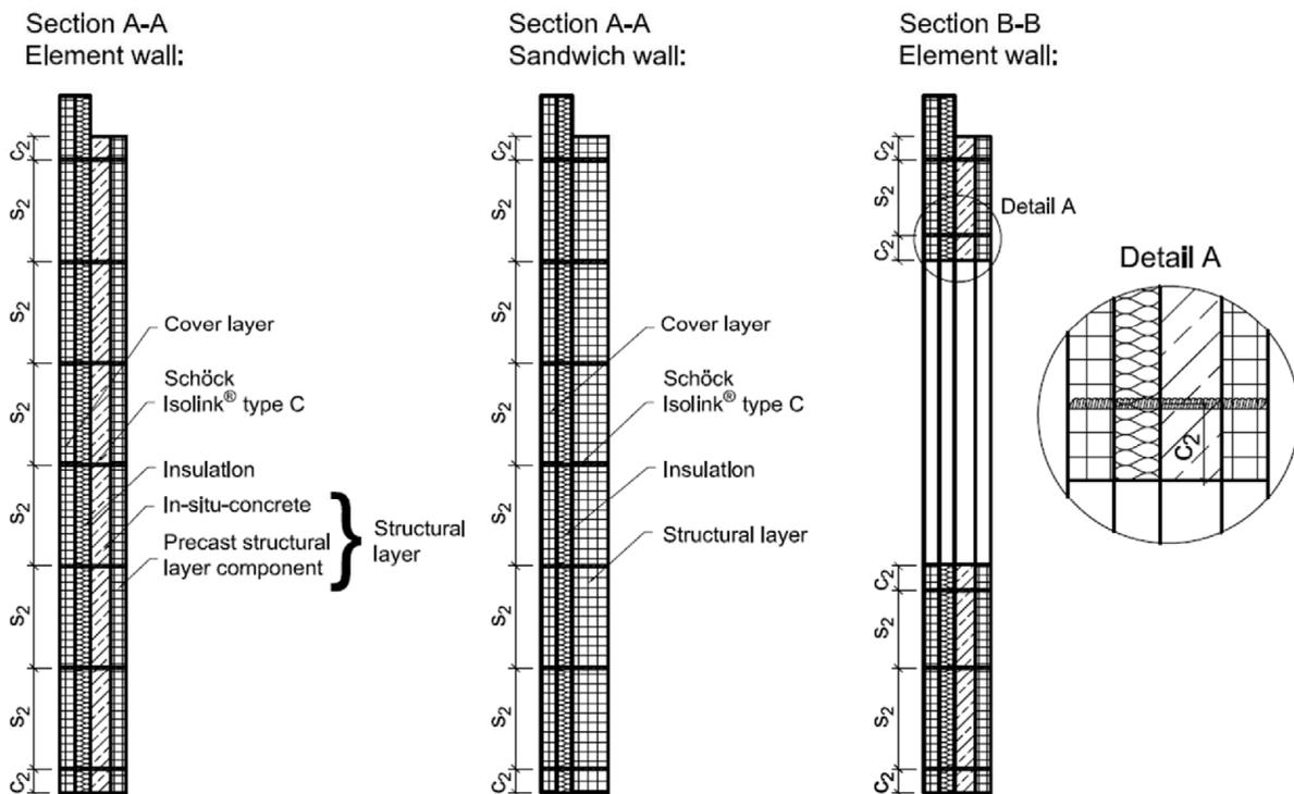
Fig. 5: Example of view of precast wall cover layer
