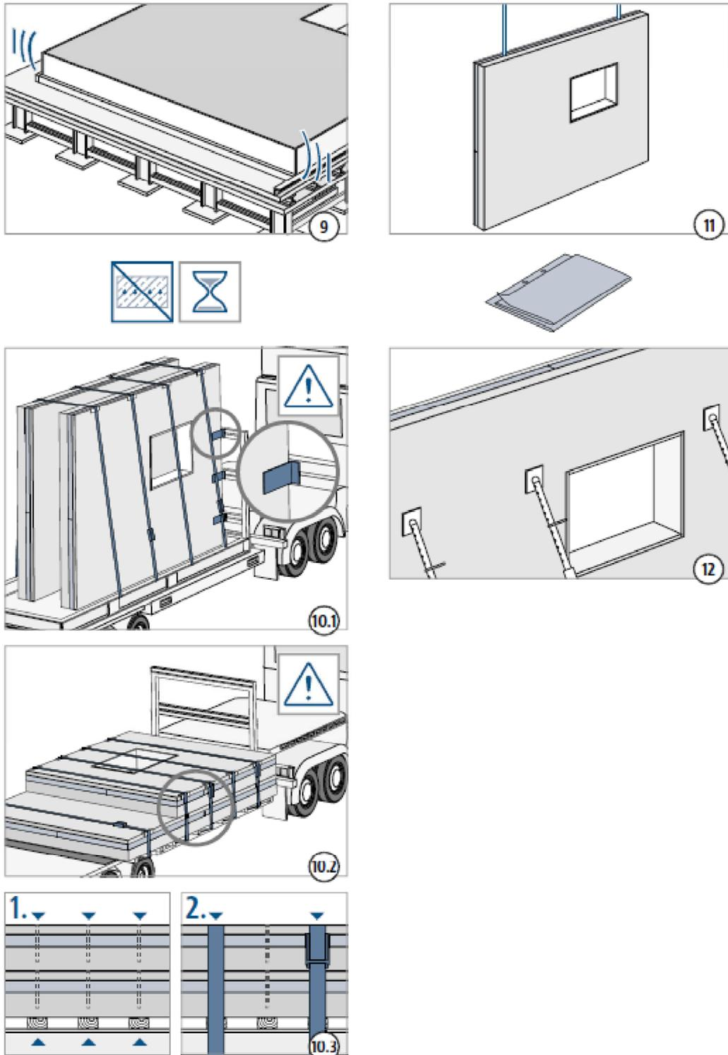
Fig. 7: Installation instruction - Schöck Isolink® for sandwich wall – page 2
