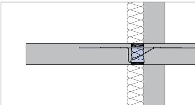
Figure 4: Assembly 2 – Balcony with thermal break element
