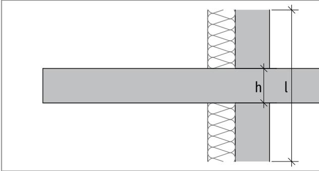
Figure 3: Assembly 1 – Balcony with thermal bridge
