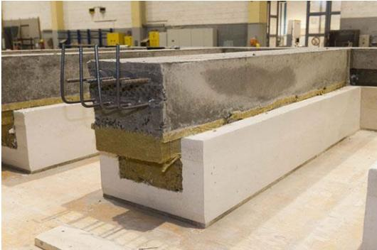
*The insulation panels in the concrete sandwich facade are up to 35 centimeters thick.*
